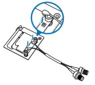
Replace the metal cover and secure the back of metal cover with the two short screws that you removed in step 1.
